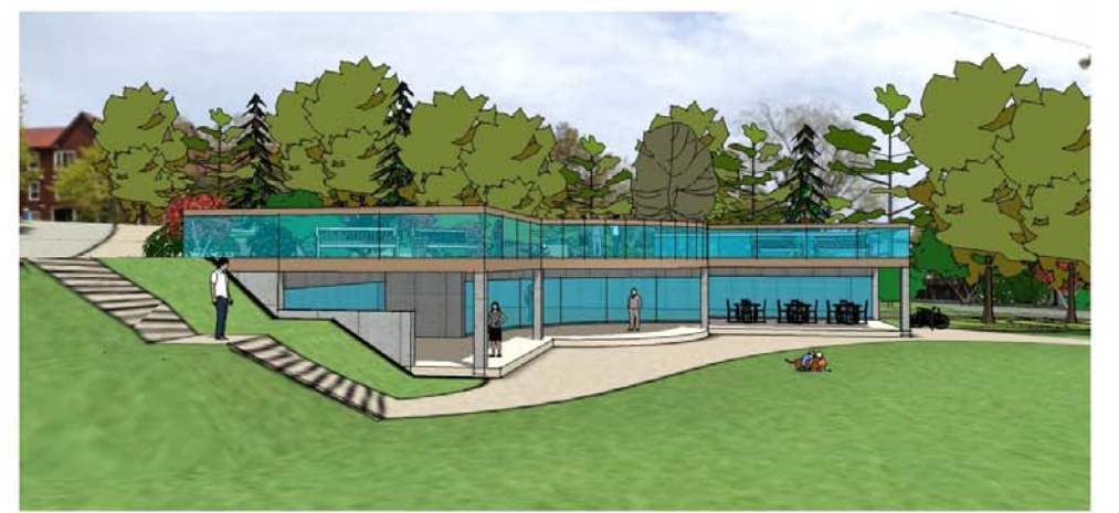
Generous overhangs for sheltered outside uses
