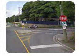
**RESTRICTIONS**: Banning possible driver movements at intersections or closing a road partially or fully to disrupt driver travel patterns. These restrictions are used to redirect traffic as well as to improve safety on a street.
